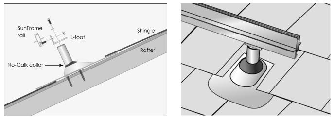
Cut an opening in the roofing material over a rafter to accommodate the flashing riser. Install the standoff, ensuring that both lag bolts are screwed into the rafter. Insert the flashing under the shingle above and over the shaft of the standoff. No-Calk collar does not require sealing of the flashing and standoff shaft.
