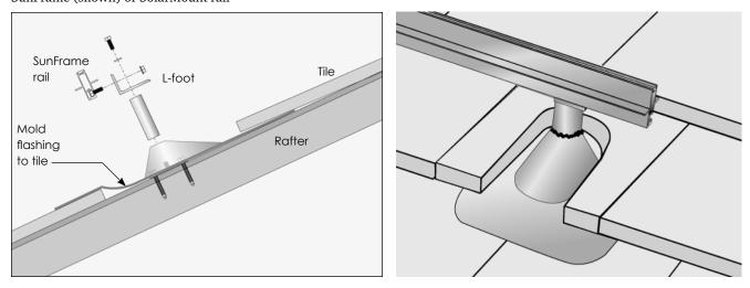
Remove a tile over a rafter. Install the base of a two-piece standoff, ensuring that both lag bolts are screwed into the rafter. Install soft aluminum flashing over the base, inserting it under the tile above and forming it to the shape of the tile. Insert standoff shaft through the opening in the flashing, screwing it down firmly in place onto the base. Seal with roofing cement or other appropriate compound.
